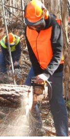
RST students learn the process of maintaining, preparing and operating hand-held chainsaws in a work environment whilst attaining their chainsaw ticket.
